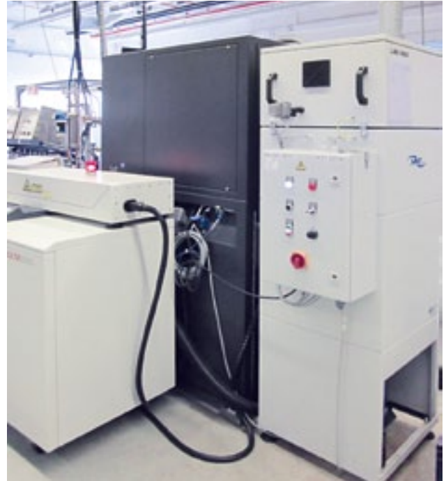
Laser welding system with integrated fume extraction system
