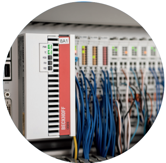
The GRS550 has a modern stepper motor controller with monitoring of all axes via encoder
